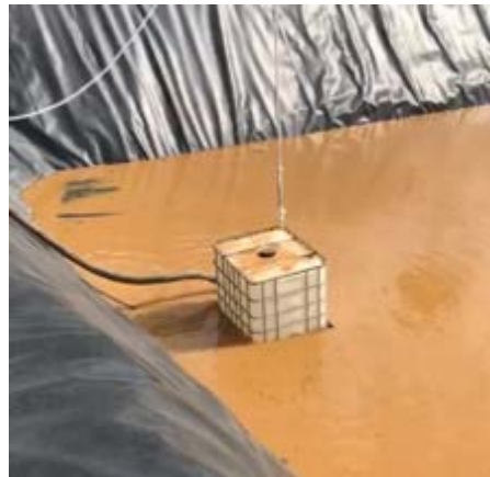
Pregnant Pond Flygt mounted under IBC Float to return solution to cells
