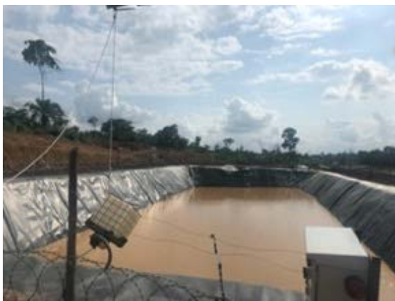
Pregnant Pond Flygt mounted under IBC Float to return solution to cells
