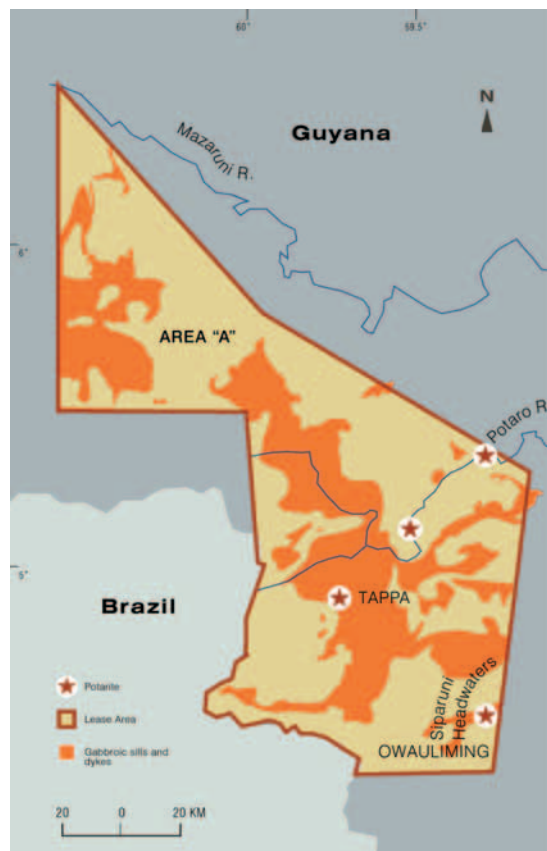
Figure 20.2 Distribution of gabbroic sills and dykes in the Roraima Group of Lease Area “A”. Note the four sites where potarite (a palladium – mercury mineral) has been collected during alluvial gold and diamond mining. Gabbro sills represent an exploration target for platinum group metals – PGMs. Source: Minter, 2002a.
