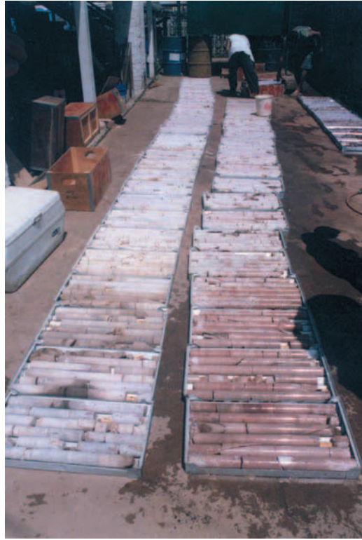
Figure 13.1 Trays of drill hole core laid out for inspection at GoldStone's core storage facility in Georgetown. The facility is equipped to provide full logistical and manpower support to GoldStone's field geologists during field mapping, sampling and exploration. Source: P Snowden.
